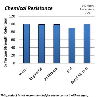
This product is not recommended for use in contact with oxygen, oxygen rich systems and other strong oxidizing materials. This product may adversely affect some thermoplastics and users must check compatibility of the product with such substrates before using.
