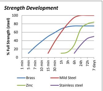
\*Cure times are typical at 23°C. Copper and its alloys will follow the faster cure while oxidised or passivated surfaces like stainless steel will tend towards the slower curve. Lower temperatures or large gaps will tend to extend the cure time. To reduce the cure time the use of Permabond A905, ASC10, or heat can be considered.
