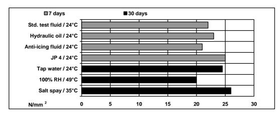
Lap shear strength versus temperature (ISO 4587) (typical average values) Cure: 42 days at 22°C
